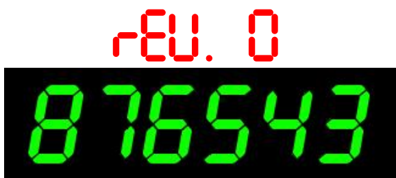
Example of normal display format displaying the number 876543
