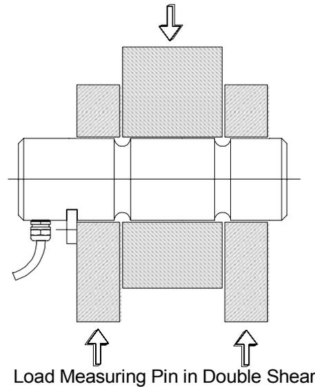
Load measuring pins are designed for many diverse applications as direct replacements for clevis or pivot pins. They have many advantages over other load sensors in that they do not normally require any change to the mechanical structure being monitored. Load pins are typically used in rope, chain and brake anchors, sheaves, shackles, bearing blocks and pivots.
