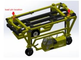
To meet the new legislative requirements, LCM Systems had to redesign the electronics of their existing system, and also introduce a new tablet display that showed the load on each individual pin and the total weight. Two existing load bearing pins were replaced with custom designed 25 tonne load measuring pins, which connect to an interface module where the mV/V output signal is converted to RS485 and the data then sent to the in-cab tablet display.
