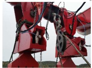
susceptible to damage. The load cells are used to sense the force of the load during a lift, and when the load exceeds a pre-set percentage of the cranes rated capacity, an overload device temporarily stops the crane from lifting and only permits the lowering of the load.
