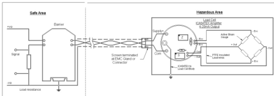
The barrier shown above limits the amount of electrical energy that can be transferred into the hazardous area, thereby preventing the ignition of a flammable atmosphere in the event of a fault condition occurring.
