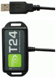
T24-BSu Wireless USB connected base station
